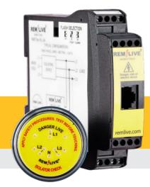
The **REMLIVE RL-24i** Isolator Check provides the user with a positive check when isolating plant. It provides electrical isolation between the DIN rail unit and the door mounted display unit. The door unit is designed to fit through the front of a control panel or switch so the user can see a live/isolation status. The super bright REMLIVE RL-24i display provides the user with a quick and easy method of proof of isolation in lock out / tag out procedures.
