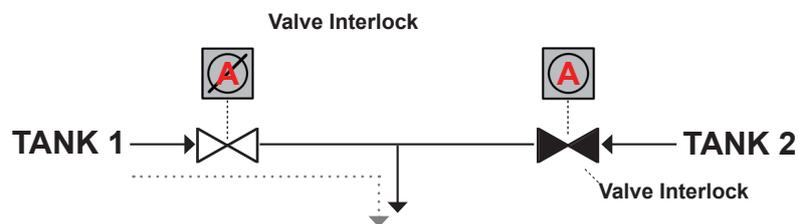
In this application, only one of the tanks can feed into the supply at once. The use of Valve Interlocks ensures only one of the lines can be open because the two interlocks share a single key. Each valve can only be opened while a key is trapped in the locked position in the lock.
