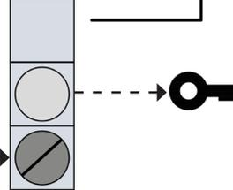
Access key trapped, Personnel (safety) key removed, Access Guard (door) open.
