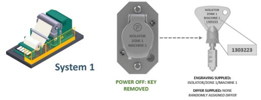
If this key were to be taken to the adjoining *System 2* where power remains live, as it has the same key code, it can be used to access the guard on the machine whilst the machine is operational. Accessing the machine in *System 2* in this state could lead to serious injury or even fatal consequences. Every measure must be taken to prevent the possibility of this duplication.
