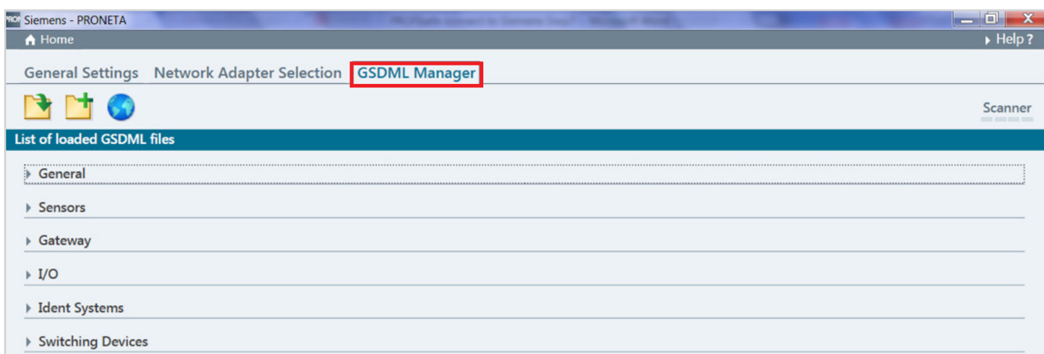
Figure 1: Open PRONETA, go to GSDML Manager Page and click on load button to add GSDML file for the first time
