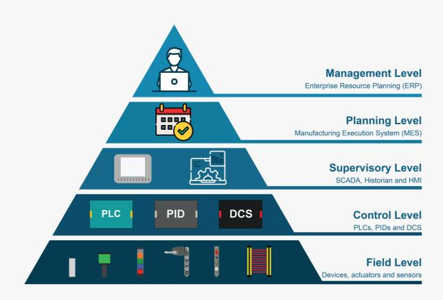
IO-Link is a means of communicating at the Field Level of the Automation Hierarchy. It has been around since 2009 and acts as a communication link between the fieldbus and the field devices.
